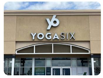
Channel letters are they are three-dimensional, individually crafted letters or logos that are typically illuminated from the inside, creating a vibrant and eye-catching sign. The illumination is usually achieved using LED lights, although neon tubing was also common in older signs.
